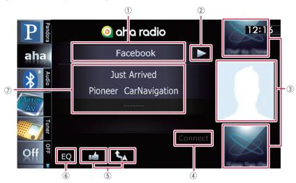
① Selects an Aha Radio station from the list Touching this key displays the list of your available Aha Radio stations. Touch the desired Aha Radio station to change Aha sources.
